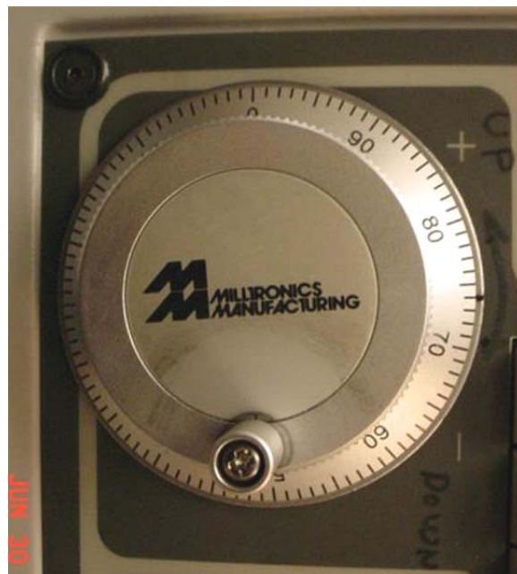
Figure 44 - Endmill position crank
