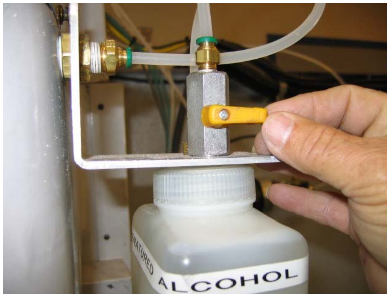
Figure 21 - Reservoir with lever at "off" (3 o'clock) position
